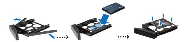
4 Insert the loaded hard drive tray into the empty hard drive bay.
