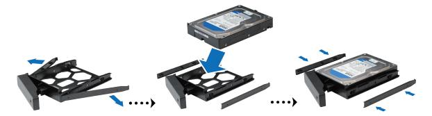
• For 2.5" drives: Remove the fastening panels from the sides of the drive tray and store them in a safe place. Place the drive in the blue area (shown below) of the drive tray. Turn the tray upside down and tighten the screws to secure the drive in place.
