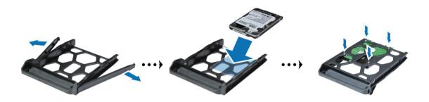
4 Make sure the side marked with **"UP"** is facing up, and insert the drive tray into the empty drive bay. You should hear a click when the tray is locked into place.
