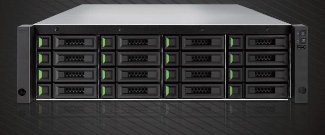
QSAN XCubeDAS XD5300 Series is a cost-effective DAS (Direct Attached Storage) or JBOD (Just a Bunch Of Disks) for server expansion. It is also a RAID expansion enclosure for QSAN SAN (Storage Area Network) XCubeSAN series.
