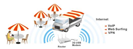
After connecting into the router, 3G USB Modem will be regarded as the third WAN port. However, the original WAN1 and WAN2 still can be used and Load-Balance can be done in the router. Besides, 3G USB Modem in WAN3 also can be used as backup device. Therefore, when WAN1 and WAN2 are not available, the router will use 3.5G for supporting
