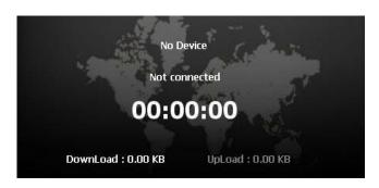
A: Make sure that the C170 Series is plugged in/inserted correctly. If it is, and No Device is still displayed, check the LED.
