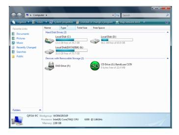
The computer treats the C170 Series as if it were a CD drive. Because of this, your computer may be trying to boot from it, as if it were expecting a Boot CD. Disconnect the C170 Series before booting.
