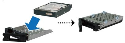
• For 2.5" drives: Place the drive in the drive tray. Turn the tray upside down and tighten screws into the four spots indicated below to secure the drive.
