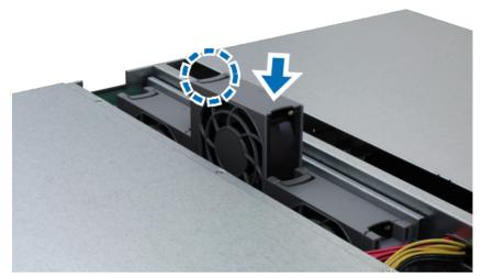
6 Put back the fan cover by reversing the remove direction of step 2.
