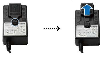
2 Slide the plug adapter provided into the slots by pushing it downward. Note that the plug adapter that comes with your DiskStation varies depending on your region. The image below is for reference only.
