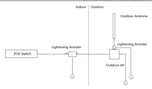
Attached Figure 1 Connect Involved Components
