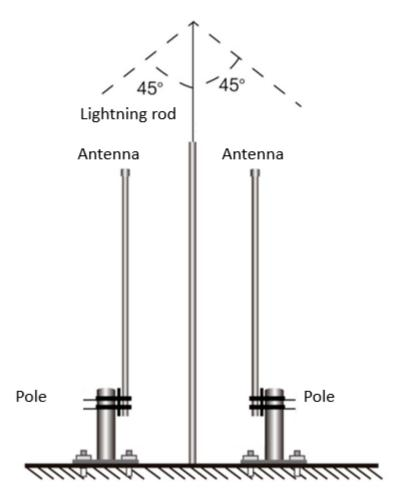
Figure 3-6 Installation of Omni Outdoor Antenna
