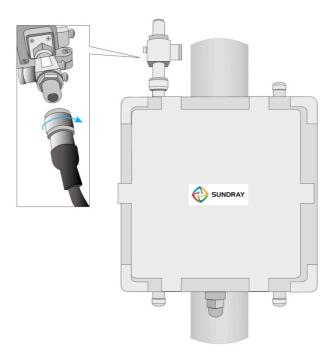
Figure 3-8 Connect RF Cable to Feeder Lightning Arrester
