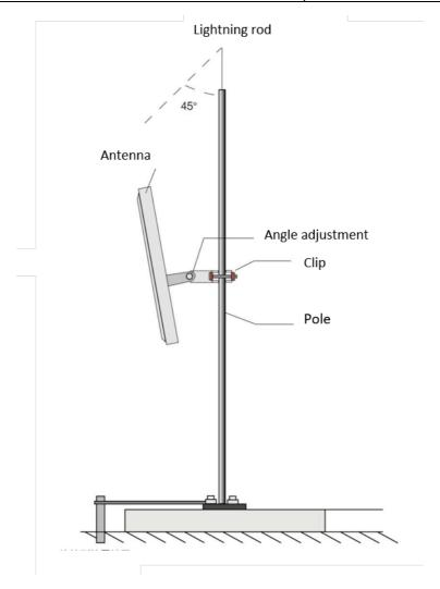
Figure 3-7 Installation of Directional Outdoor Antenna
