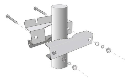
Figure 3-2 Install Bracket on a Pole
