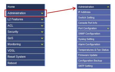
"Administration" section is for users to manage the MINI IP DSLAM, including the IP address, switch settings, etc. It includes the following detail functions.
