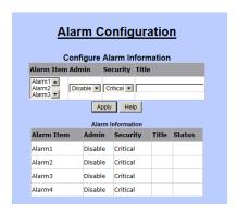
"Alarm Configuration" is distinguished into two tables: Configure Alarm Information and Alarm Information.
