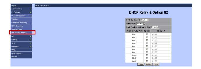
"DHCP" stands for "Dynamic Host Configuration Protocol", which is a network protocol that is for configuring network devices dynamically so these devices can communicate on an IP network. It is a service that runs at the application layer of TCP/IP protocol stack to assign IP addresses to its clients dynamically.
