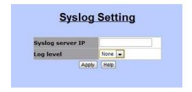
"Syslog" function is supported in this MINI IP DSLAM system. The system will send logs to a remote log system. In this system, three events will be reported to the remote log system: cold start, warm start and link change. The followings are necessary for connecting the remote syslog server.
