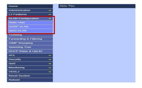
The MINI IP DSLAM supports three kinds of VLAN algorithms:
