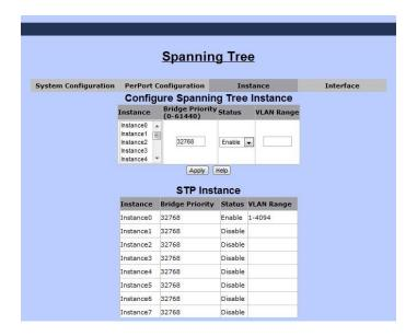
"Instance" function is a part of MSTP function. MSTP allows users to map a group of VLANs into a single Multiple Spanning Tree Instance (MSTI). This means the spanning tree protocol is applied separately for a set of VLANs instead of the whole network.
