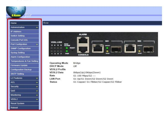
"Menu" section is located on the left hand side of the page and users are allowed to change the configuration and review the status of the device by interacting this section.
