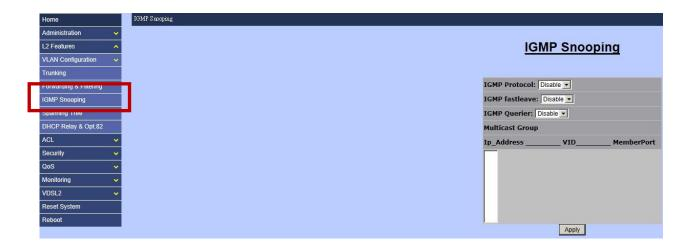
"IGMP" stands for "Internet Group Management Protocol". IGMP allows hosts and routers to build multicast group memberships. IGMP snooping presents the process of IGMP network traffic listening. With this feature, MINI IP DSLAM is able to listen to IGMP conversation between hosts and routers. The switch is able to maintain a relation map of links and IP multicast streams.
