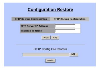
Users are able to load or backup configurations via "Configuration Restore" function. This function includes two tabs: "TFTP Restore Configuration" and "TFTP Backup Configuration".
