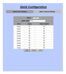
QinQ VLAN function allows users or service providers to separate traffic service for different customers by adding service provide VLAN tags and customer VLAN IDs. In this function, settings are divided into two parts:
