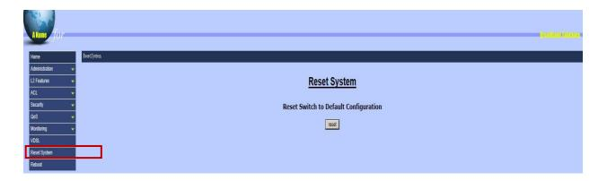
"Reset System" is for restoring all configurations back to the default factory configurations. All the settings will be changed back to the original state.
