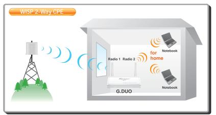
Traditionally, the WISP operators will need 2 access points to provide total wireless access for their subscribers. That means one AP to outdoor and one AP for subscriber's home wireless network. Not only this increases the deployment cost, it also consumes more energy and complicates the installation. G.DUO's "WISP+AP" wireless operation mode is specially designed to satisfy WISP operator's requirement. The Site Survey wizard combines AP scanning,
