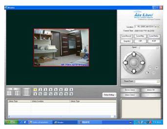
The CamPro Express allows you to monitor 16 channels via the computer and WEB UI. You can choose how you would like to view the camera, the Cam Pro Express supports 1/4/9/16 different view. You can also choose to view the different camera in single view or 1/4/9/16 view.
