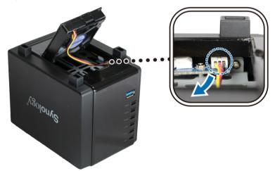
4 Remove the screws from the fan case and slide out the malfunctioning fan.
