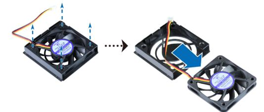
5 Slide a new fan into the fan case. Tighten the screws to secure the fan in place.
