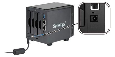
**3** Connect at least one LAN cable to one of the LAN ports of the DiskStation. Connect the other end to your switch, router, or hub.
