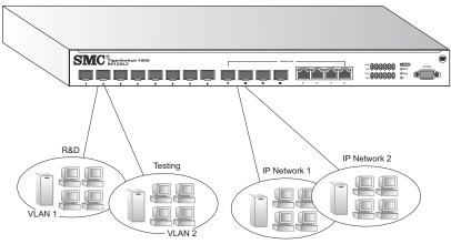
Figure 2-5. IP Routing for Unicast Traffic
