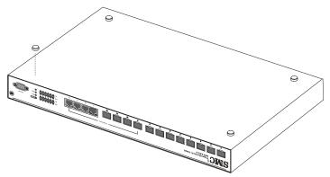
Figure 3-4. Attaching the Adhesive Feet
