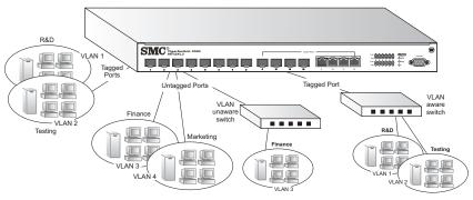
Figure 2-4. Making VLAN Connections
