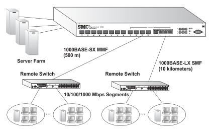
Figure 2-3. Remote Connection with Fiber Cable
