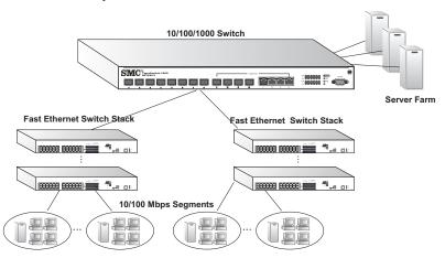
Figure 2-2. Central Wiring Closet
