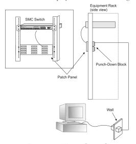
Figure 4-2. Wiring Closet Connections
