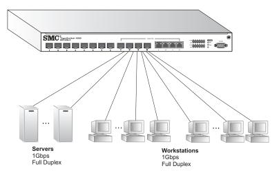
Figure 2-1. Collapsed Backbone
