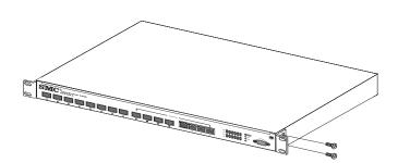
Figure 3-2. Attaching the Brackets
