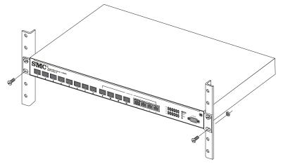
Figure 3-3. Installing the Switch in a Rack
