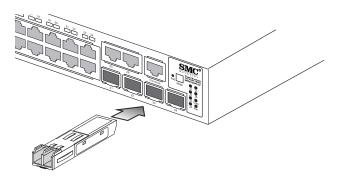
Figure 3-5 Inserting an SFP Transceiver into a Slot
