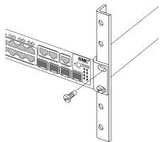
Figure 3-3 Installing the Switch in a Rack
