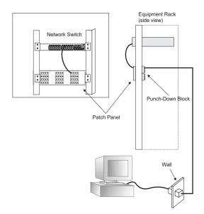
Figure 4-2 Network Wiring Connections
