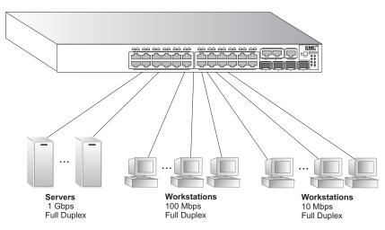
Figure 2-1 Collapsed Backbone
