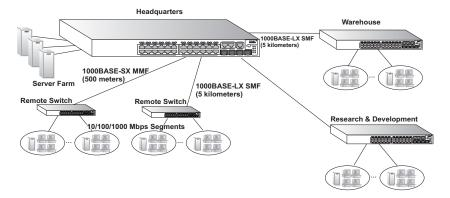
Figure 2-3 Remote Connections with Fiber Cable
