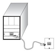
Figure 4-1 Making Twisted-Pair Connections
