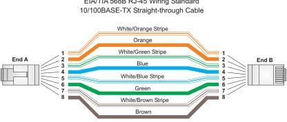
EIA/TIA 568B RJ-45 Wiring Standard
