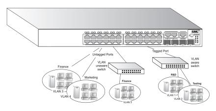
Figure 2-4 Making VLAN Connections
