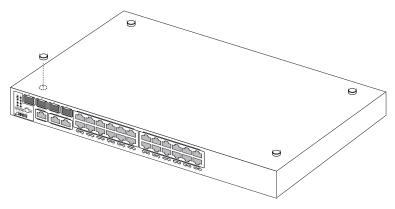
Figure 3-4 Attaching the Adhesive Feet
