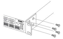
Figure 3-2 Attaching the Brackets
