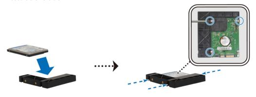
**b** Slide the 2.5" Disk Holder into the hard drive bay, and push it all the way until the hard disk is firmly connected to the SATA connector. Secure the Disk Holder with the provided screws.
