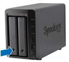
2 Pull the drive tray handle in the direction indicated below to remove it.
