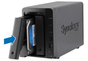
5 Insert the included tray key into the tray lock. Turn the key clockwise (to the "I" position) to lock the handle. Remove the key.
