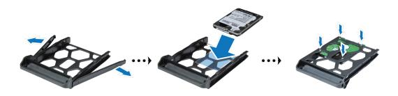
**4** Make sure the side marked with "UP" is facing up, and insert the drive tray into the empty drive bay. You should hear a click when the tray is locked into place.
