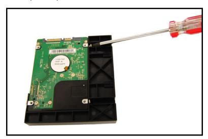
Slide the 2.5" Disk Holder into the hard disk bay and push it all the way back until it is connected to the SATA connector. Secure the Disk Holder with the 2 hard disk screws provided.
