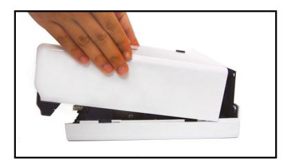
6. Secure the case with the 2 case screws provided.
