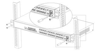
Figure 3-2 Installing the switch on the cabinet
