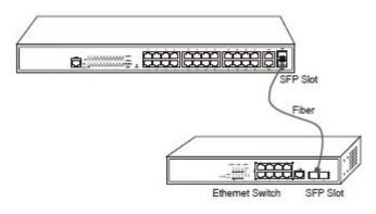
Figure 3-6 Gigabit optical ports and other switches
