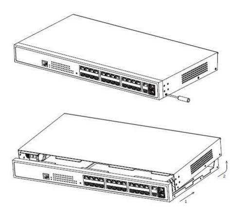
Figure 4-1 Opening the chassis of S2226PB
