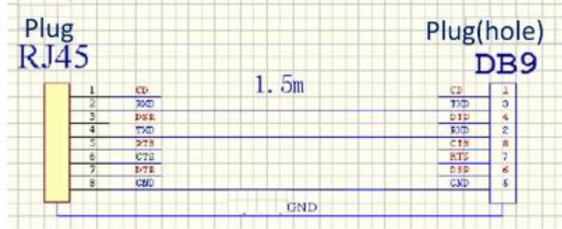
Figure 3-5 Cable connection at the console port
