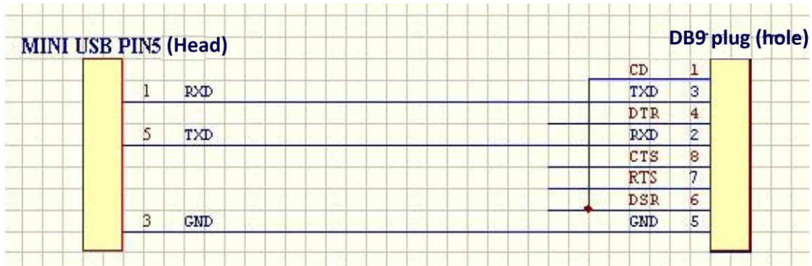
Figure 3-4 Cable connection at the console port
