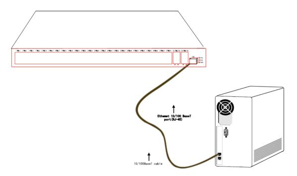
Figure 3-3 Connecting the console port of BDCOM S2928E switch and computer
