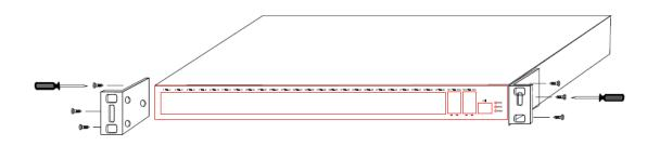
Figure 3-1 Fixing the machine box of the switch
