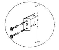
Figure 3-2 Installing the switch on the cabinet
