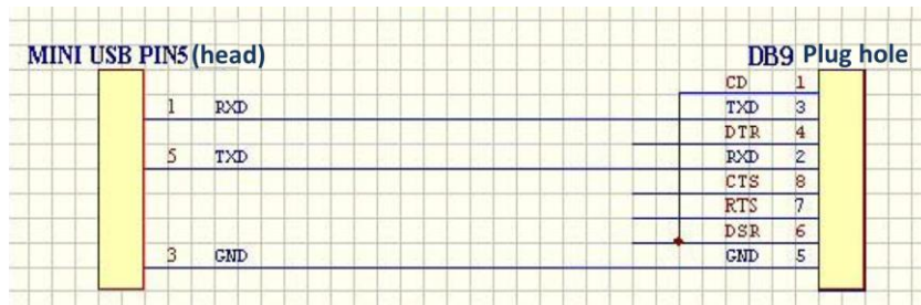
Figure 3-4 Cable connection at the console port
