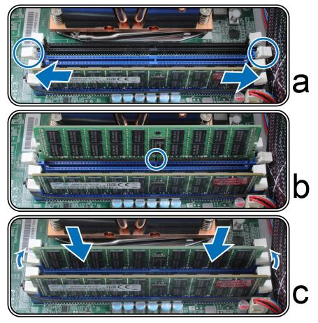
Note: Hold the memory module by its edges, and do not touch the gold connectors.
