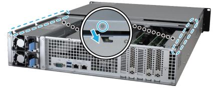
b Put back and fasten the screw you removed in step 2-a.
