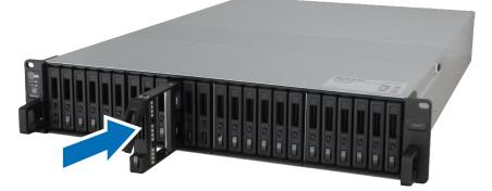
Note: Make sure the tray is pushed in all the way. Otherwise, the drive might not be able to function properly.
