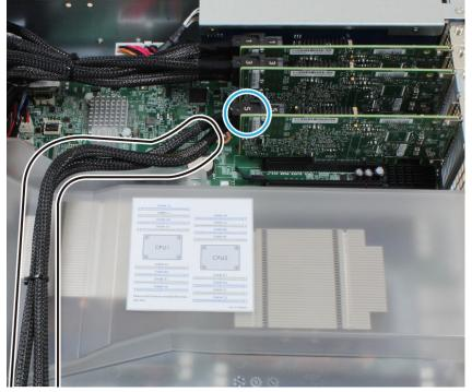
5 Remove the 3 screws that secure the ventilation duct cover, pull up the ventilation duct cover, and put it aside.
