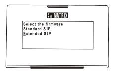
The phone will start loading the Extended IP Phone Firmware. It will display current firmware being loaded.
