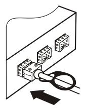
Insert the connector into the slot
