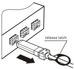
Pull the release latch to remove
