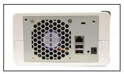
2. Push the upper case forward to slide it open. Lift the upper case and set it aside.
