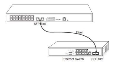
Figure 3-7 Connecting the SFP ports and other Ethernet terminals
