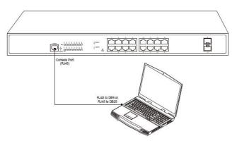
Figure 3-4 Connecting the console port of S2518PB and computer
