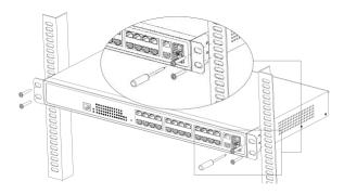
Figure 3-2 Installing the switch on the cabinet
