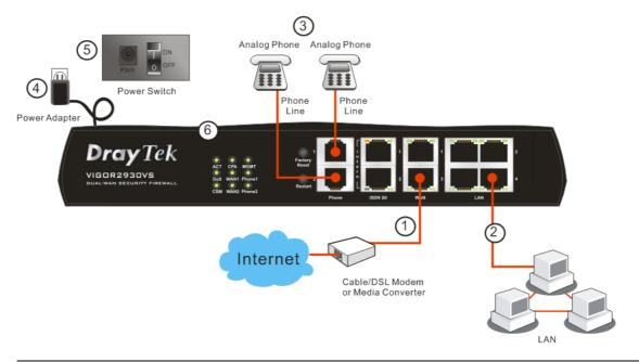
**Caution**: Each of the Phone ports can be connected to an analog phone only. Do not connect the phone ports to the telephone wall jack. Such connection might damage your router.
