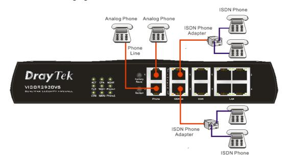
Yet, if the user configures ISDN S0 2 as TE Mode in **VoIP>> Phone Settings**, the **green** LED will light on to indicate **ISDN2-TE** is selected. Then, the port is specified for ISDN line only. Refer to the following figure for reference.
