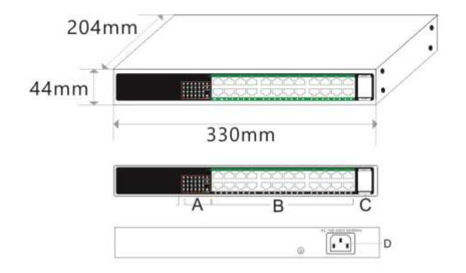
A.Working indicator B.24\*PoE ports C.2\*1000M uplink SFP ports D.power input portAC100-240V,50-60Hz
